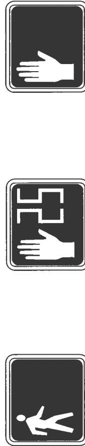
PERSON WALKING INTERVAL FLASHING UPRAISED HAND INTERVAL STEADY UPRAISED HAND INTERVAL LED COUNTDOWN PEDESTRIAN SIGNAL FACE MODULE DETAIL B
