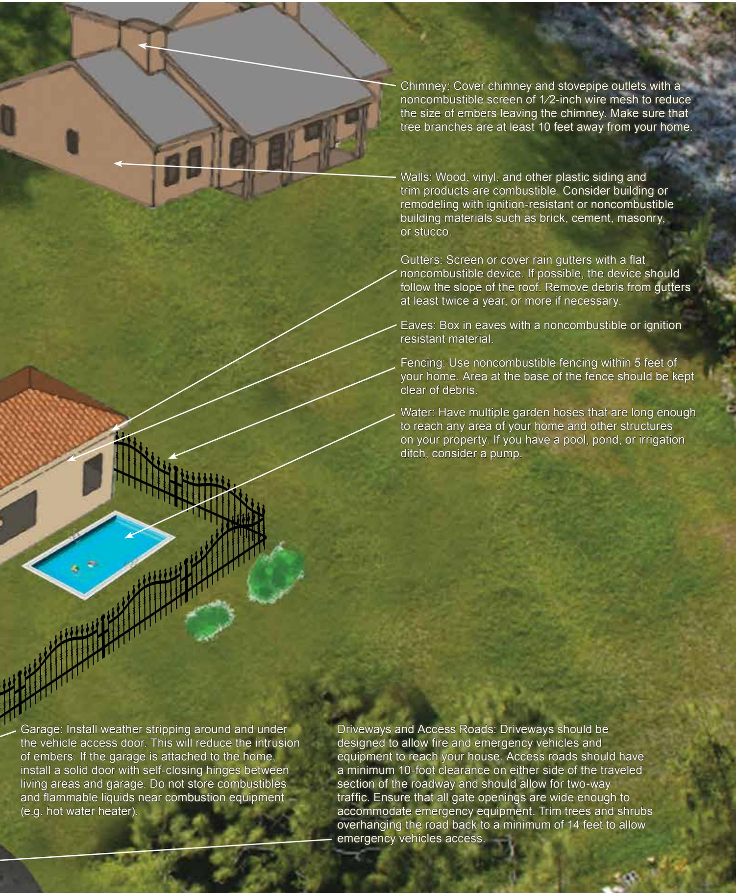
**Chimney:** Cover chimney and stovepipe outlets with a noncombustible screen of 1/2-inch wire mesh to reduce the size of embers leaving the chimney. Make sure that tree branches are at least 10 feet away from your home.
